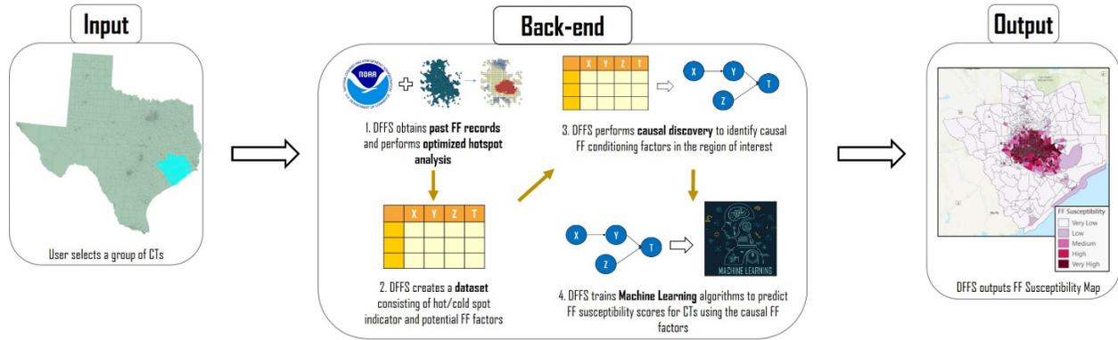
Fig 1: Methodology of the Dynamic Flash Flood Susceptibility (DFSS) tool
